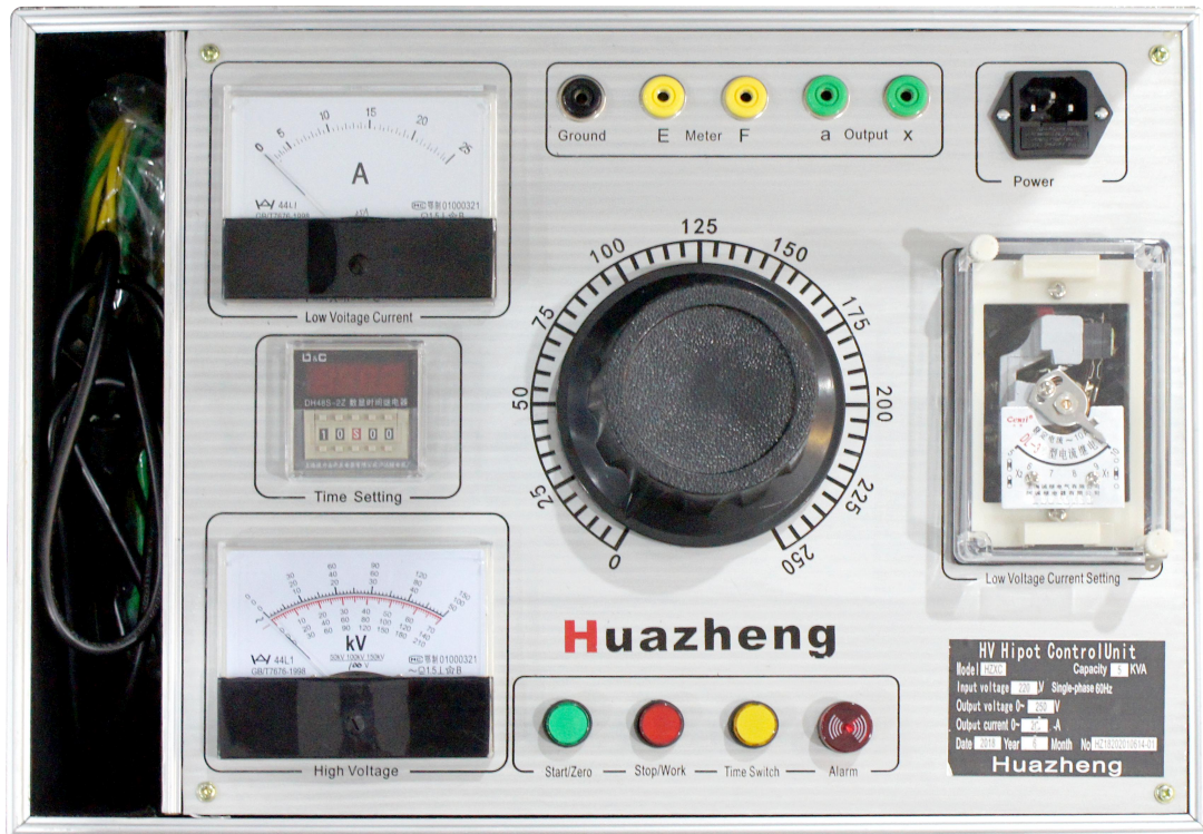
Figure 4 Panel of main control box
